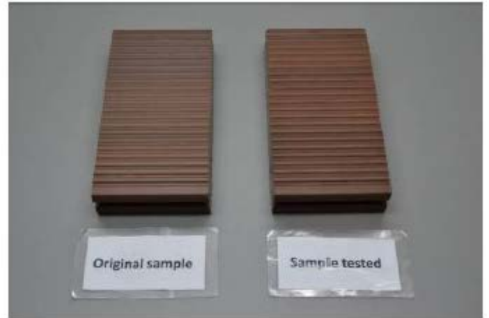
Model: US02. After 1500 h test, Gray Scale=4, \Delta E^*=1.60
