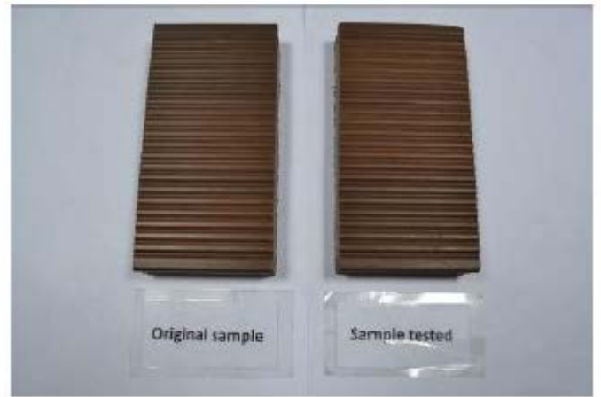
Model: US02. After 1000 h test, Gray Scale=4-5, \Delta E^*=1.33 .
