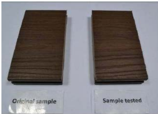
Model: US01. After 500 h test, Gray Scale=4-5, \Delta E^*=0.65
