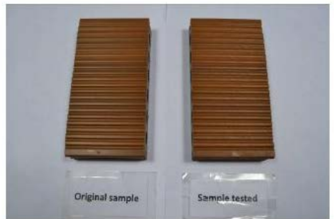
Model: UH07. After 1000 h test, Gray Scale=4-5, \Delta E^*=1.41 .
